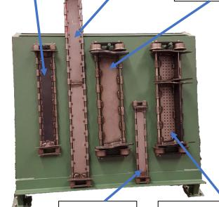
24 Inch 2 ½" Pitch Standard Pan 24 Inch 6" Pitch Flush-top, perforated, two-lane, flanged Wheel Belt Pan 30 Inch 9" Pitch Standard Belt Pan
